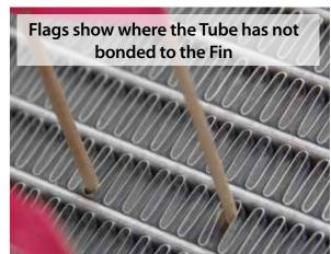
Poor brazing causes defects in fin-totube bonding, reducing heat transfer and compromising overall radiator performance.
