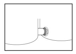
Fasten the rubber adaptor with a hose clamp
