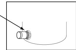
Attach the other Spigot fitting to the opposite tank closer so the rubber adaptor is connecting both tanks
