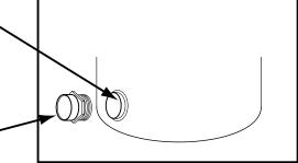
Apply thread tape to the thread
