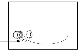
Screw the Spigot fitting into the tank
